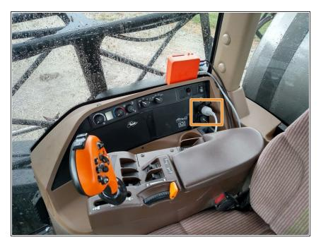
Press cable firmly into Diagnostic
